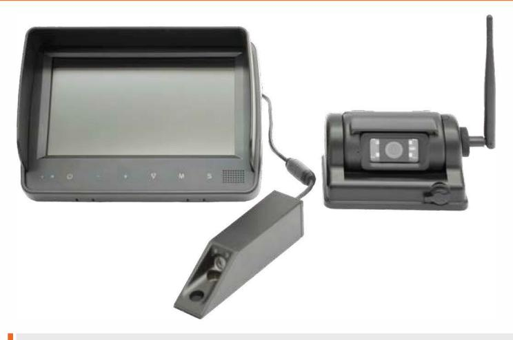
**SafeViewWireless** provides maximum positioning flexibility. With its magnetic base it can be installed on the forklift without invasive interventions. It is equipped with internal battery and charge indicator.
