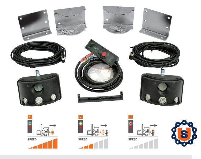
**Safe&Stop+**, suiting to vehicles wider than 1,5m, immediately alert the operator through visual and acoustic alerts. Detection is based on a pair of CySens sensors installed in the rear part of the vehicle. In addition the system can intervene on the speed of the vehicle (\*) in two steps strongly reducing the risk of collision and accident.
