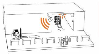
**SafeTraffic**, in its minimum configuration, is made by a sensor (installed in proximity of the area to surveil), an alert unit and a main control unit.
